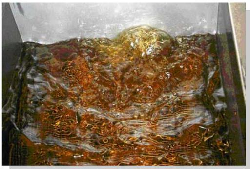
**13** Add oil if necessary to bring level to upper fill mark in frypot. Turn the fryer on to continue cooking.
