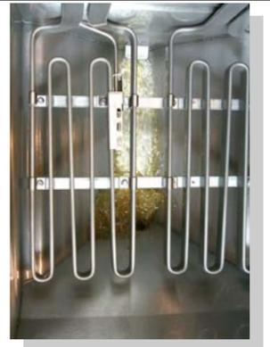
**12** The frypot will fill. As the filter pan empties, oil will bubble in the frypot. Leave the pump on for 10-15 seconds after bubbles appear to clear drain lines; turn the pump off.
