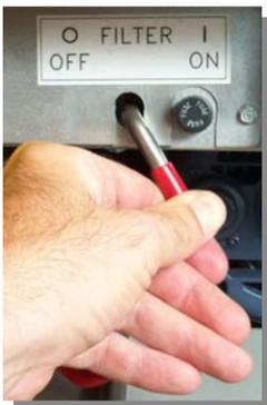
**10** Oil flows through the frypot. Allow oil to flow for 5 minutes. The frypot can be cleaned during this time.
